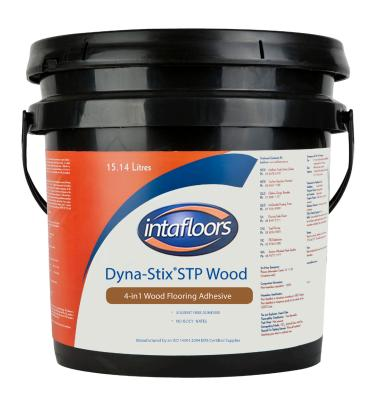
**Dyna-Stix STP Wood** is a 4-in-1 silane terminated polymer adhesive (designed for use on high moisture slabs) for the installation of multi-ply engineered wood, high-density fiber board core wood and acrylic impregnated wood plank, as well as finished and unfinished solid wood flooring (approved in writing by the wood flooring manufacturer for glue down installations), parquet and bamboo over properly prepared substrates.
