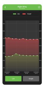
Touch the "Graph" button at the bottom of the screen with the list of readings for an individual sensor to navigate to a new screen that displays the sensor's RH and temperature data in a color graph.
