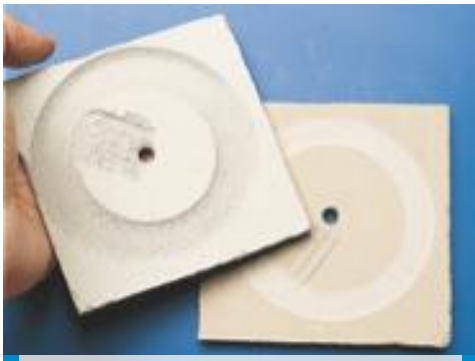
Taber abrasion executed on Ultraplan (right specimen) and on conventional levelling (left specimen) after 200 cycles
